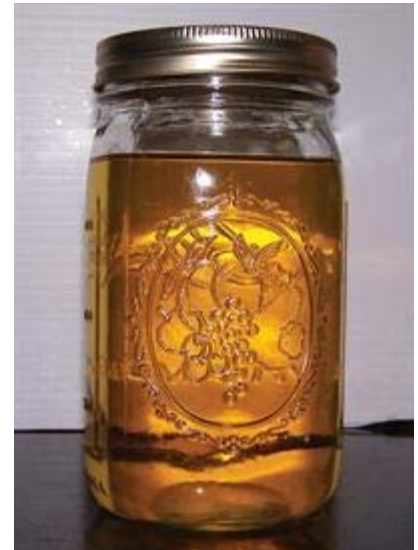
Conversion to biodiesel (transesterification) results in a liquid fuel. (Photo by Gary A. Breitenbeck)
